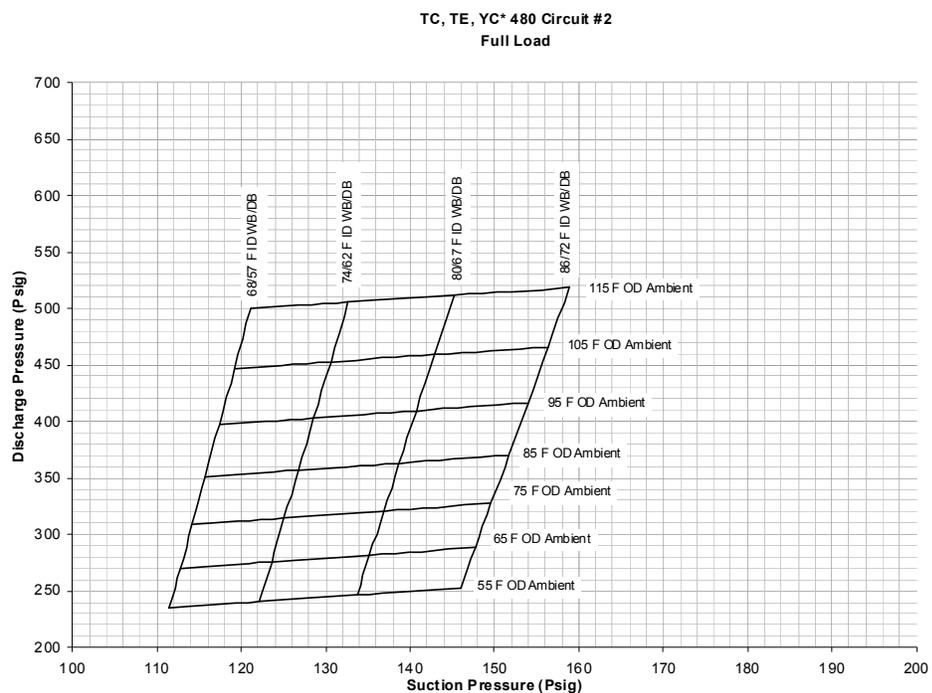
**Table 56. 50 Ton Dual Circuit—Operating Pressures (60 Hz)**
