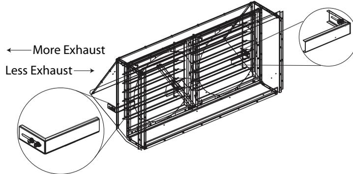
**Figure 50. (Horizontal) Standard Exhaust Maximum Damper Position**
