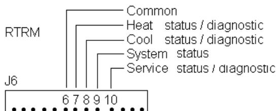
1. Measure and record DC voltage from J6-6 (common) to each output: J6-7, J6-8, J6-9, and J6-10.
