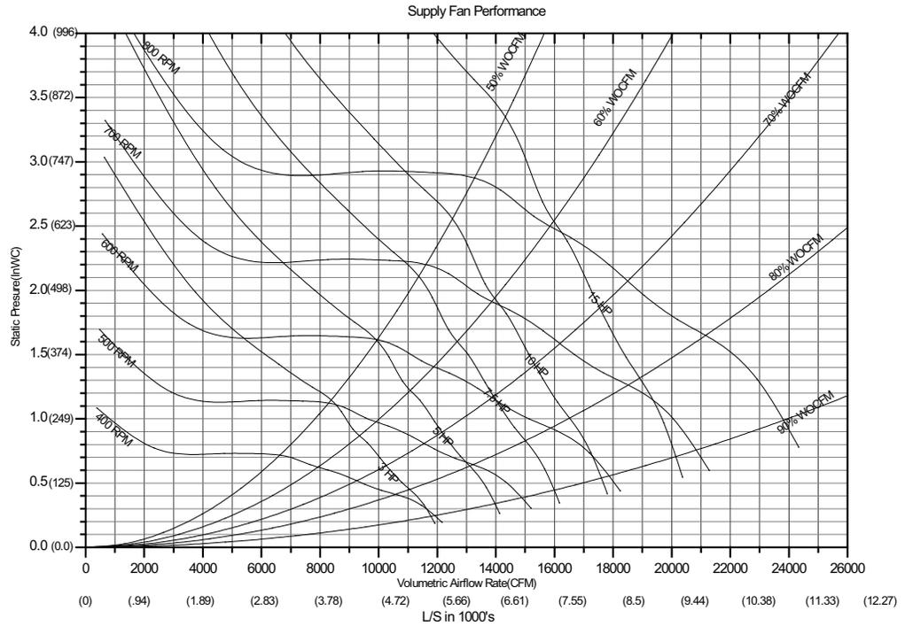
**Table 33. Supply Fan Performance—82-105 kW (SI)—50 Hz**
