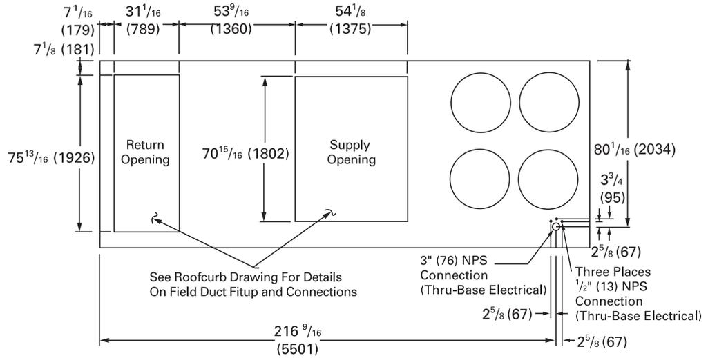
**Figure 8. Duct openings, 60 Hz 40-50, 50 Hz 33-42 Tons (TC, TE, YC Low and High Heat)**
