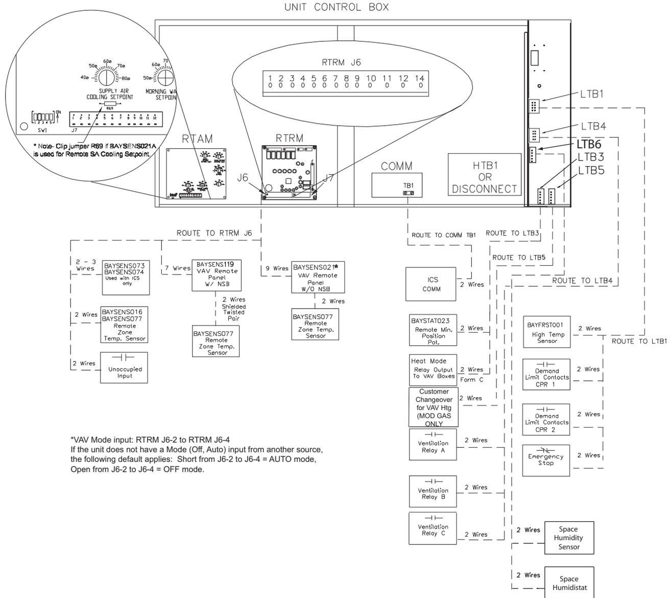
**Figure 21. RTRM Zone Sensor/Thermostat Connections**
