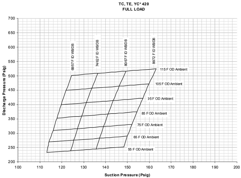
**Table 54. 40 Ton Dual Circuit—Operating Pressure (60 Hz)**
