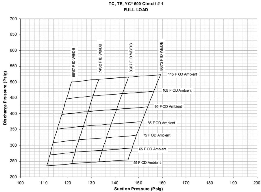
**Table 57. 50 Ton Dual Circuit—Operating Pressures (60 Hz)**
