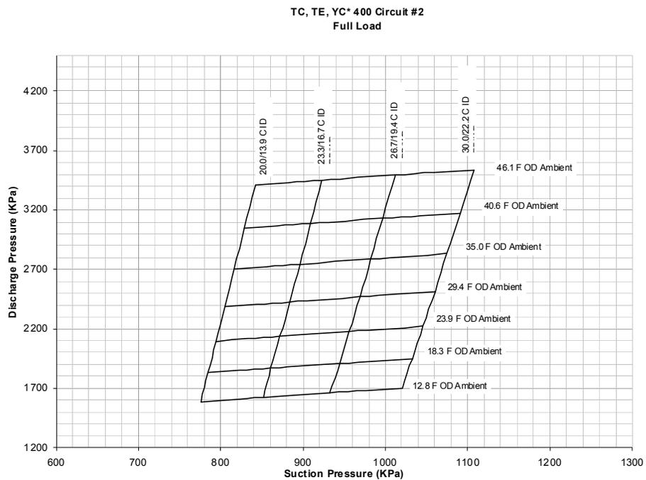
**Table 63. 41.7 Ton Dual Circuit—Operating Pressures (50 Hz)**
