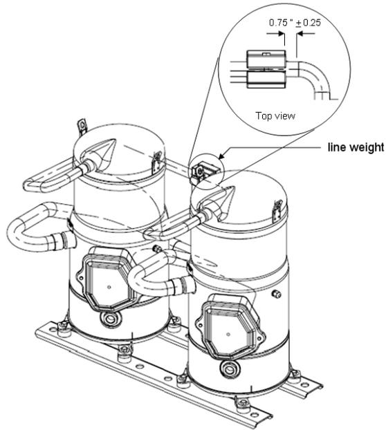
**Figure 54. Line Weight Locations—40 Ton**
