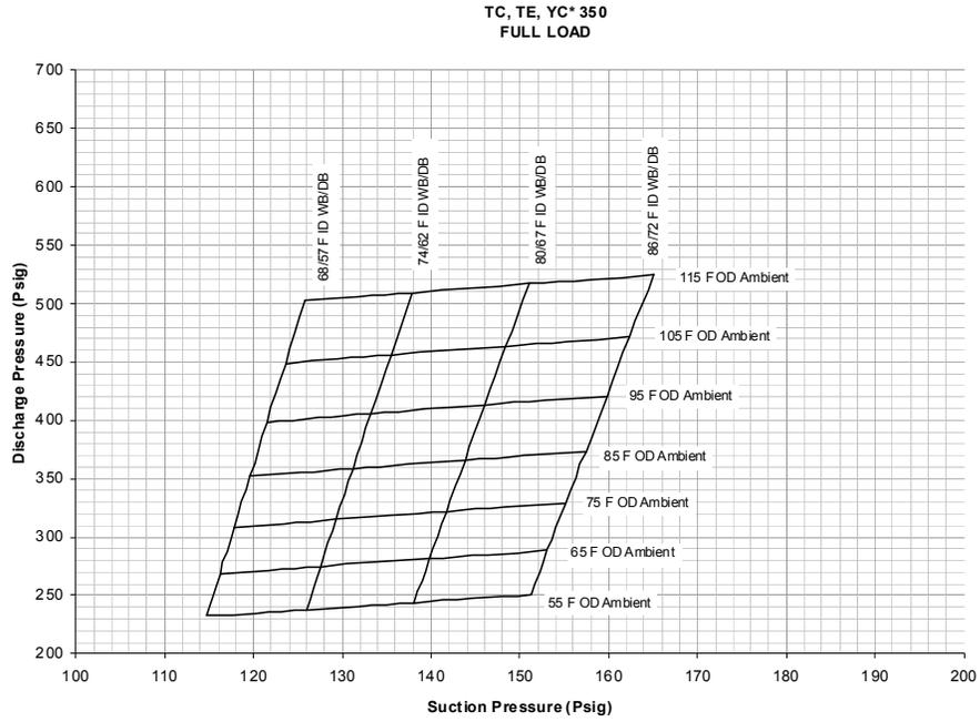
**Table 61. 33.3 Ton Dual Circuit—Operating Pressure (50 Hz)**
