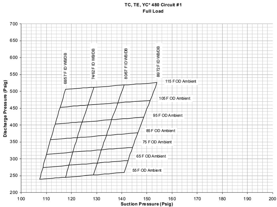
**Table 55. 40 Ton Dual Circuit—Operating Pressure (60 Hz)**
