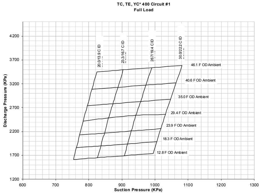
**Table 62. 33.3 Ton Dual Circuit—Operating Pressure (50 Hz)**
