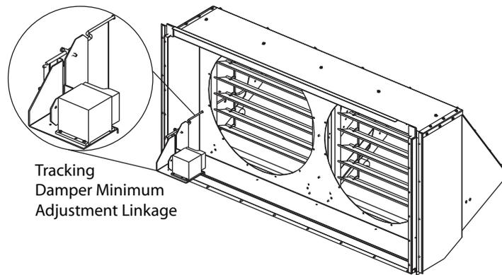
**Figure 48. (Horizontal) Tracking Exhaust Damper Adjustment**
