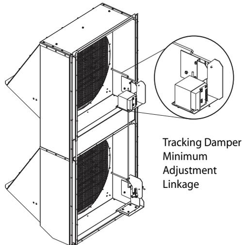
**Figure 49. (Downflow) Standard Exhaust Maximum Damper Position**
