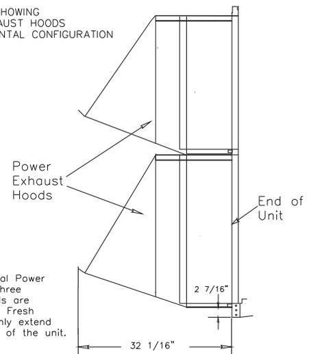
NOTE: The Two Horizontal Power Exhaust Hoods and the three Horizontal Fresh Air Hoods are located side by side. The Fresh Air Hoods (not shown) only extend 23 15/16" from the end of the unit.
