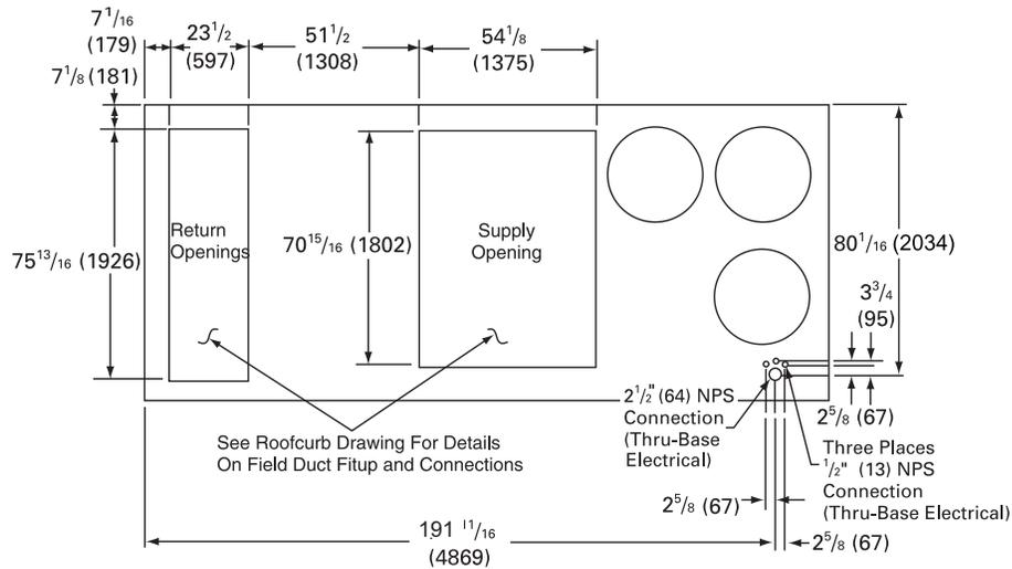
**Figure 5. Duct openings, 60 Hz 27½-35, 50 Hz 23-29 Tons (YC High Heat)**
