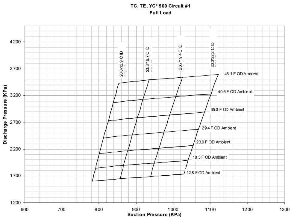
**Table 64. 41.7 Ton Dual Circuit—Operating Pressures (50 Hz)**
