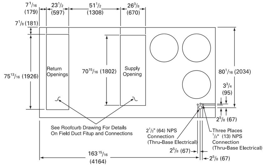
**Figure 2. Rear view showing duct openings for horizontal units**
