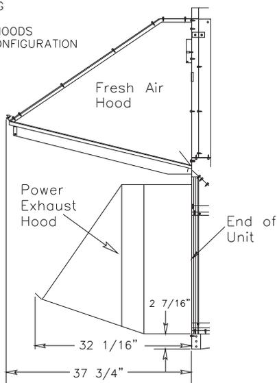
SIDE VIEW SHOWING POWER EXHAUST HOODS FOR HORIZONTAL CONFIGURATION
