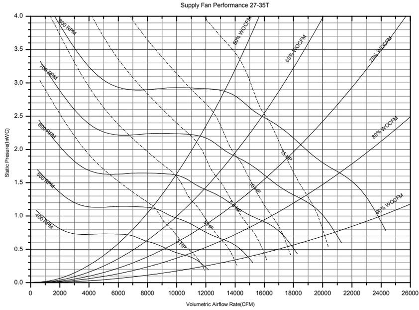
Figure 44. Supply Fan Performance Curves 40 and 50 Ton—60Hz
